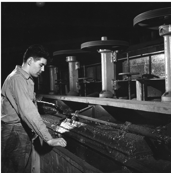
Figure 6: Flotation cells. Hector Tremblay monitoring the froth. ( NWT Mining Heritage Society – George Hunter Collection )
